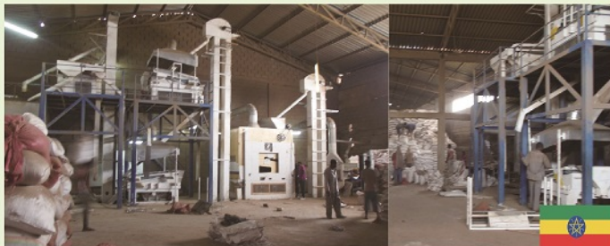
10T/H Pulses and Sesame Cleaning Plant in Ethiopia
