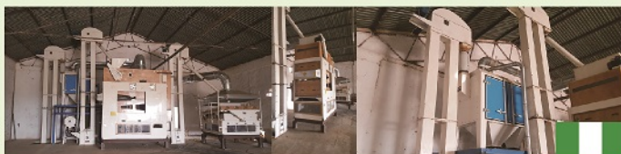
10T/H Sorghum Cleaning Plant in Nigeria
