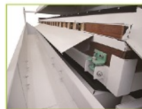
Vibrating passway for collecting the good seed
